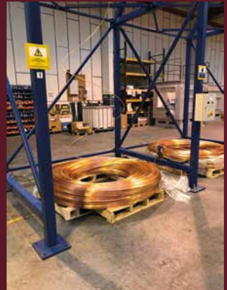
Copper Feed: 8mm CuOF Rod 送铜杆：8mm CuOF 铸杆
