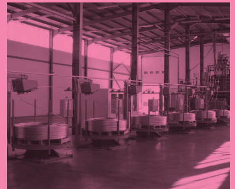
Image 3 - Rautomead RS 3000 integrated melting and Casting machine. 6 strands, 5,500 – 6,000 tonnes/year
