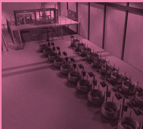
Image 4- Rautomead RDG 360 copper rod casting machine. 32 strands, 28,000 - 30,000 tonnes/year
