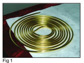
7mm diameter as cast 24 ct Gold Bonding Wire Rod
