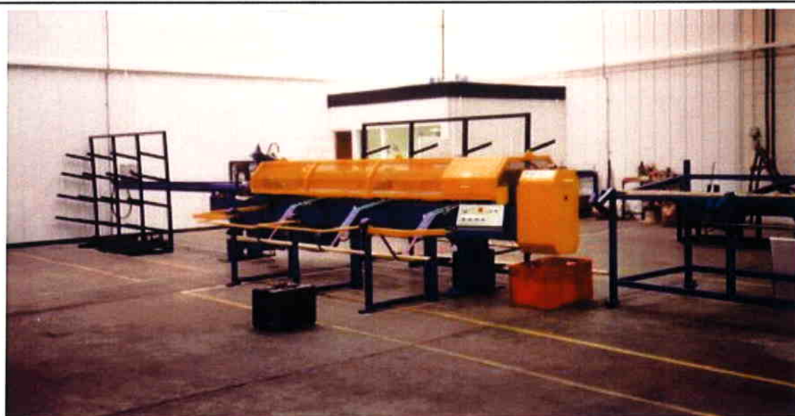
Fig 12 30 Tonne Hydraulic Shave Bench
